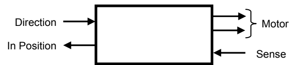
Figure 3 Turnout control circuit
