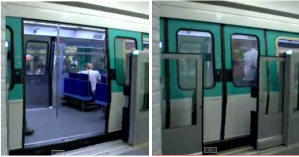
Figure 2: On the right, automatic opened doors, on the left, the platform doors are automatically closing (images extracted from youtube)
