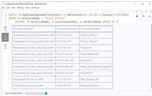
Figure 4: Result of query to find all references for the function Start_Offset in Neo4j.
